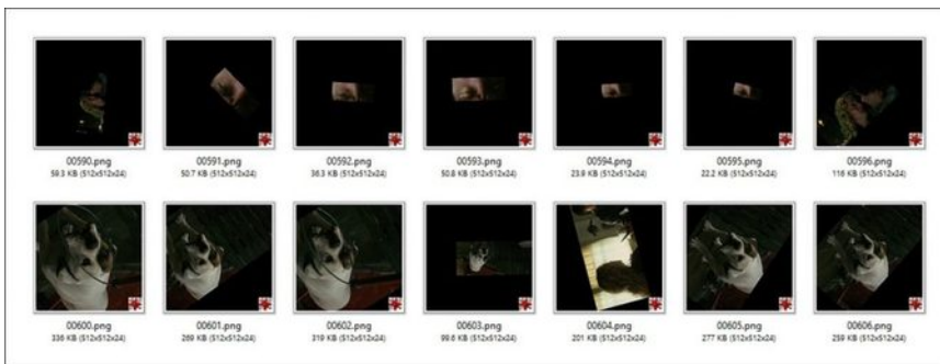
Some typical facial recognition failures in FaceSwap's extraction processes, also common to DFL. These will need to be identified and removed from the dataset before training begins.
