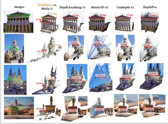
Comparison of metric-scale landmark reconstruction. Ground-truth measurements from Google Maps are shown in the left column. Across unseen real-world landmarks, WildMoGe produces scale estimates more closely matching known dimensions, while MoGe-2, DepthAnything V3, and Metric3D V2 frequently underestimate the size of distant structures. UniDepth V2 often yields more plausible scales, but remains inconsistent, whereas DepthPro occasionally produces severe scale errors.
