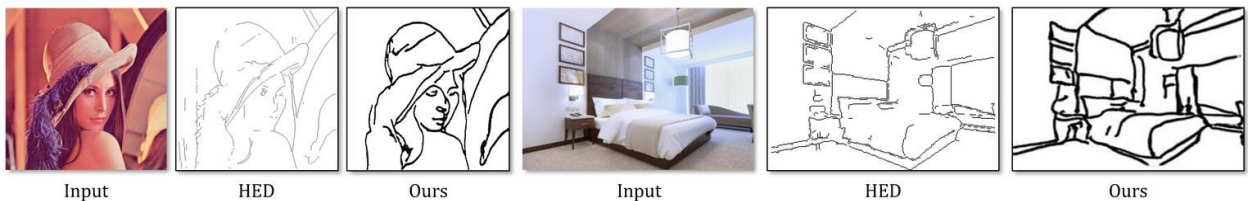
PhotoSketch uses AI-driven boundary detection to infer contours for a sketch-like equivalent to an input photo. Output from the project’s trained models and default algorithms can help train new machine learning systems to recognize and categorize domains, objects and segmented sections of objects (such as faces), and subsequently associate those labels with images. ( https://github.com/mtli/PhotoSketch )
